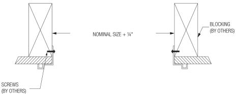
Step 3: Place the grille in the opening and using the #8 screws provided by Price, screw the grille into place using the countersunk screws.
